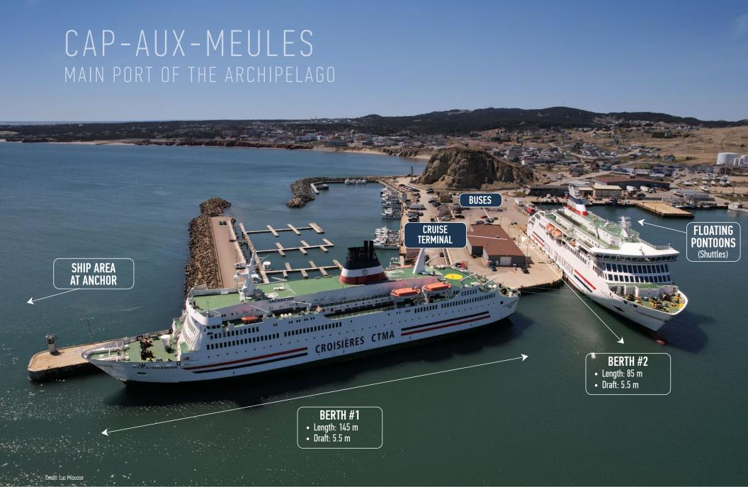
The port of Cap-aux-Meules can be reached via a channel dredged to a varying depth of 5.4 m to 6.8 m. Ships with greater draft can anchor in the Baie de Plaisance opposite the port. Anchorage sites are 1 to 1.5 nautical miles from the port, where water shuttles can easily dock.
